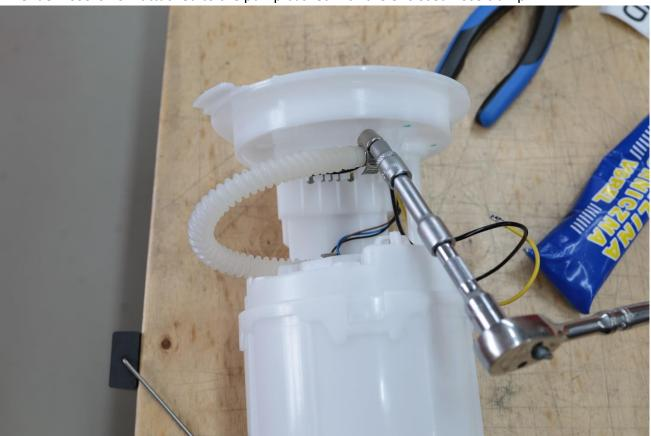
**11.** Now the cables are plugged back into the pump while paying attention to the cable routing it should now look like this:
